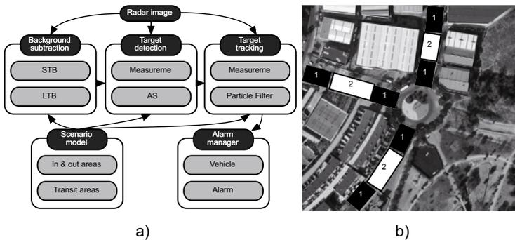
**Fig. 1.** a) Software architecture overview and b) expert knowledge modeling of a roundabout with in & out (1) and transit (2) areas
