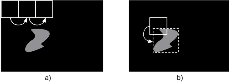
**Fig. 3.** Adaptive Sliding Window movement (left) and local search when the window detects part of a foreground object (right)
