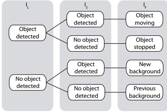
**Fig. 2.** Event detection using dual background subtraction
